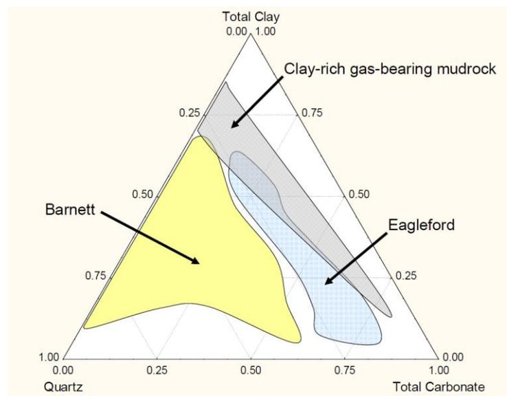
Mineral composition is variable in shale gas reservoirs. (Passey et al., 2010)
