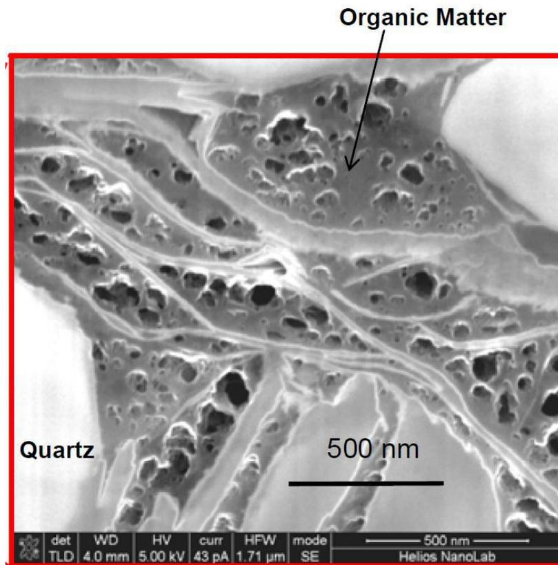
Pores seen on SEM photomicrograph of a Barnett organic-rich rock containing gas. (Passey et al., 2010)
