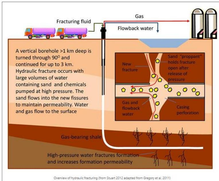
Shale gas extraction involves drilling of deep horizontal boreholes and enhancing the natural permeability of the shale by hydraulic fracturing ("fracking"). Fluid is introduced to raise the downhole pressure above the fracture pressure of the formation rock creating fissures and interconnected cracks that increase the permeability of the formation. Fracking is used to overcome
